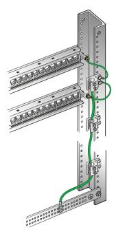
Figure 5: Panels grounded to earthing terminals, then to the telecommunications grounding bus-bar
