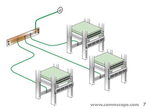
Figure 6: Earthing and bonding of equipment cabinets and racks
