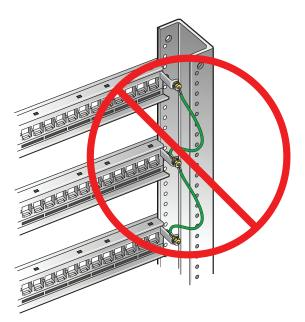
Figure 3: Daisy chaining of ground straps is not allowed
