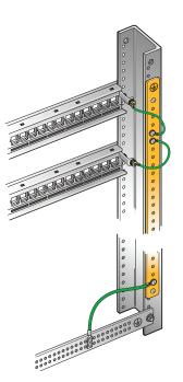
Figure 4: Use of Vertical **Grounding Bus-Bar**
