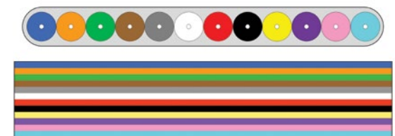
Conventional Flat Ribbon Matrix (Side View and Top View)
